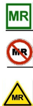
Figure 1: ASTM Standard F2503 for Making Medical Devices and Other Items for Safety in the Magnetic Resonance Environment. From top to bottom the symbols for MR safe, MR unsafe and MR conditionally safe.
